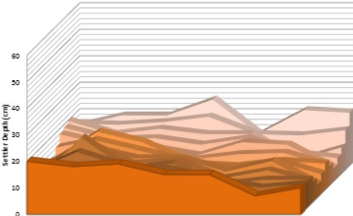
Figure 6. Settler bottom solids profile before Crud Forx application.
