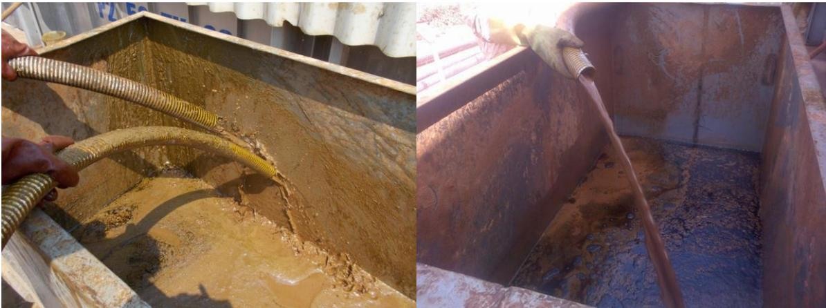
Figure 5. Typical Crud Forx bottom solids slurry discharge into crud barrow.
