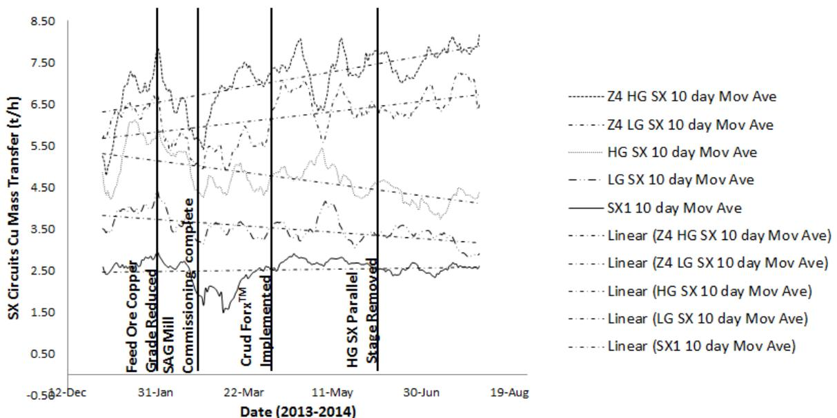
Figure 9. Mutanda SX circuits copper mass transfer (Dec 2013 to August 2014).
