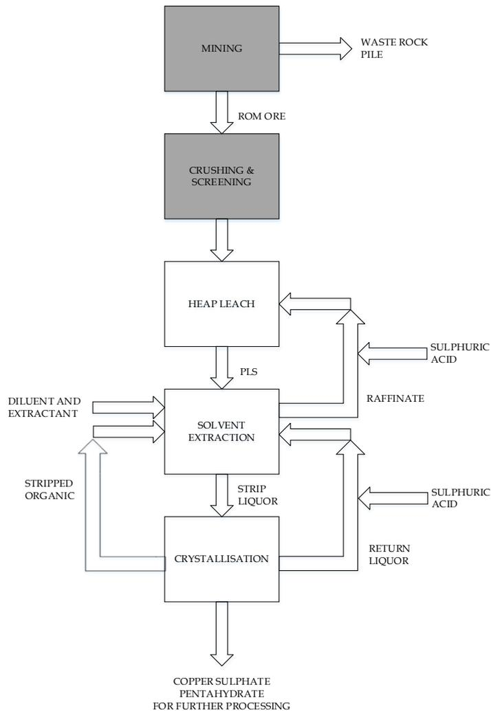
Figure 2. Copper sulphate crystallisation process simplified flowsheet.
